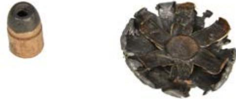
Figure 3: A .44 magnum bullet is stopped within three layers of Kevlar XP.
