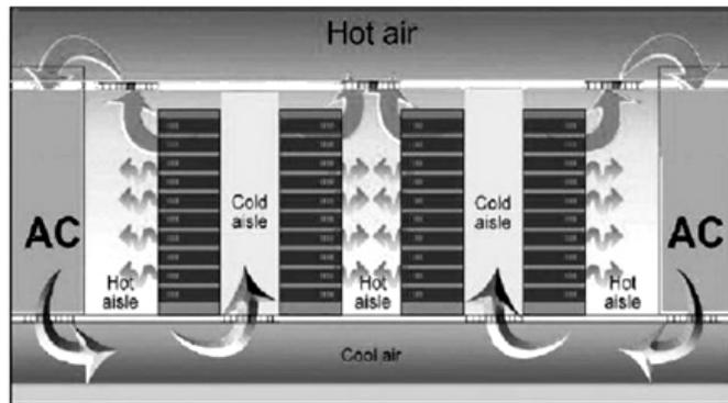
Figure 3: Typical air flow in a traditional data center.
