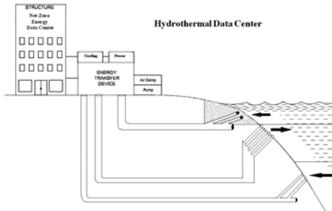
*Figure 4: The above illustrates the concept of a large data center using tunnel boring and directional drilling to access and discharge cold and warm seawater or lake water. The cold water will be used for cooling the data center. Turbines and heat exchangers will generate clean electric power by utilizing the temperature difference of warm surface water and deep cold water. This power is used to*
